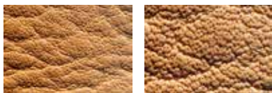
Pure aniline leather: the pores are clearly visible, there is no color coating applied to the leather.
