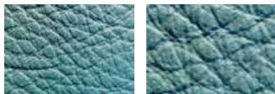
Pigmented smooth leather: the pores are hardly visible, a thick layer of dye has been applied to the leather.
