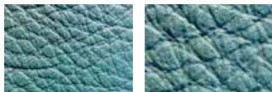
Pigmented smooth leather: the pores are hardly visible, a thick layer of dye has been applied to the leather.
