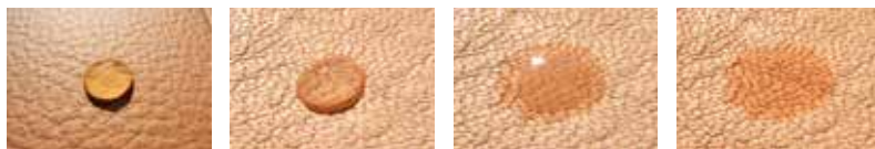
Picture 1 shows a drop of water on pigmented cowhide. The water doesn't penetrate the leather.
