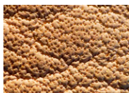
Pure aniline leather: the pores are clearly visible, there is no color coating applied to the leather.
