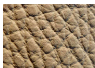
Pigmented smooth leather: the pores are no longer recognizable, a thick layer of dye has been applied to the leather.
