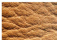
Pure aniline leather: the pores are clearly visible, there is no color coating applied to the leather.
