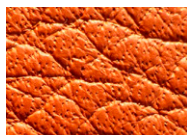
Semi-aniline leather: the pores are clearly visible, but a thin layer of dye has been applied to the leather.
