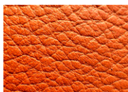
Semi-aniline leather: the pores are clearly visible, but a thin layer of dye has been applied to the leather.
