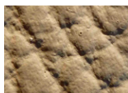
Pigmented smooth leather: the pores are no longer recognizable, a thick layer of dye has been applied to the leather.
